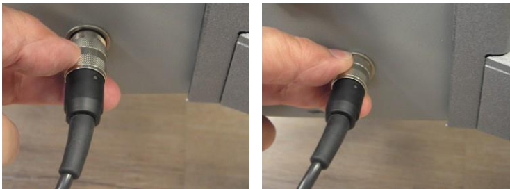
Figure 3-25. Connecting the Left Footswitch's Cable to its Connector on the System's Rear Side
