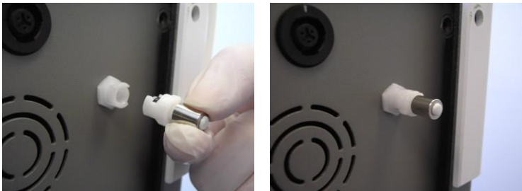
Figure 3-86. Connecting the Luer Lock Air Cap to the System's Air Outlet Port #2
