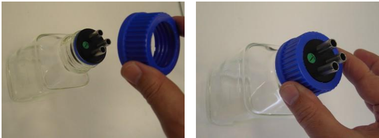
Figure 3-34. Closing the Jar's Lid
