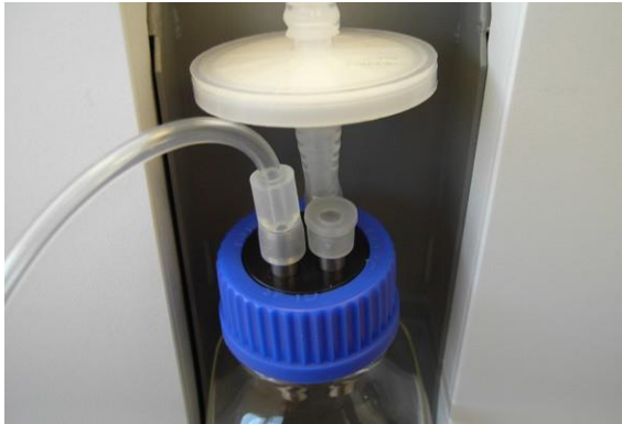
Figure 3-62. Silicon Cap Connected to the Waste Jar's Unused Inlet Pipe
