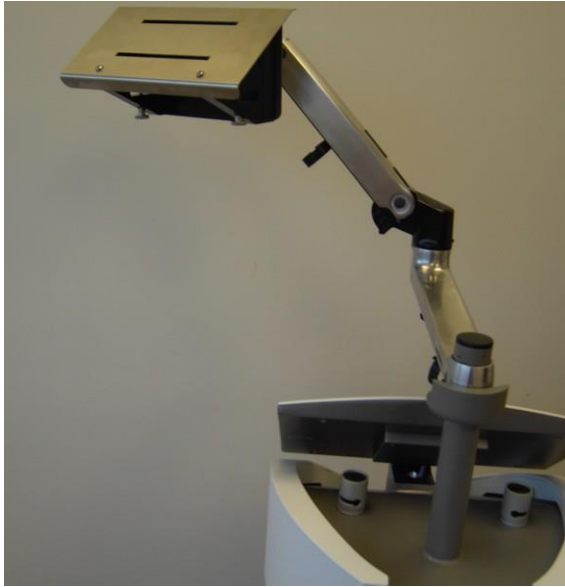
Figure 3-13. Handpiece Tray Installed
