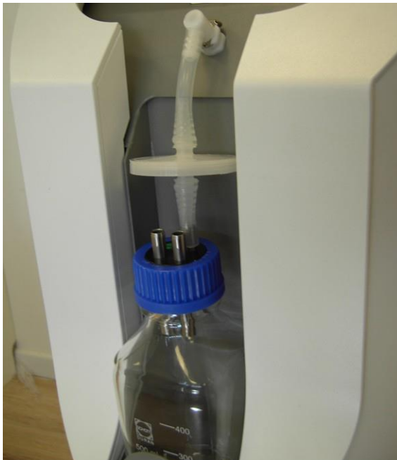
Figure 3-44. Filter Assembly Installed
