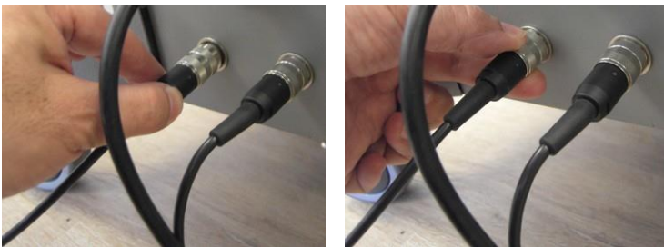
Figure 3-29. Connecting the Right Footswitch's Cable to its Connector on the System's Rear Side
